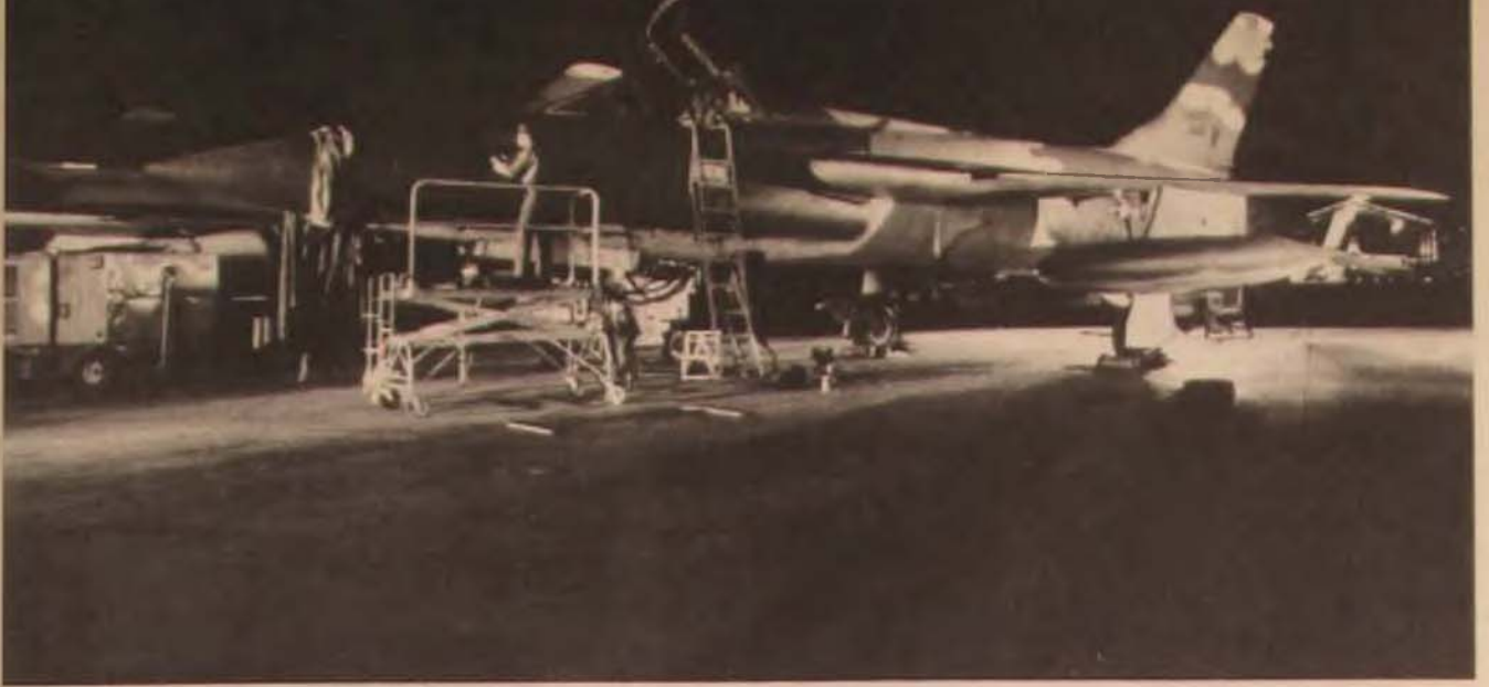
After the Seventh Air Force F-105 has been released by maintenance section, quality control technicians recheck the work performed on the airframe to insure greater safety.
