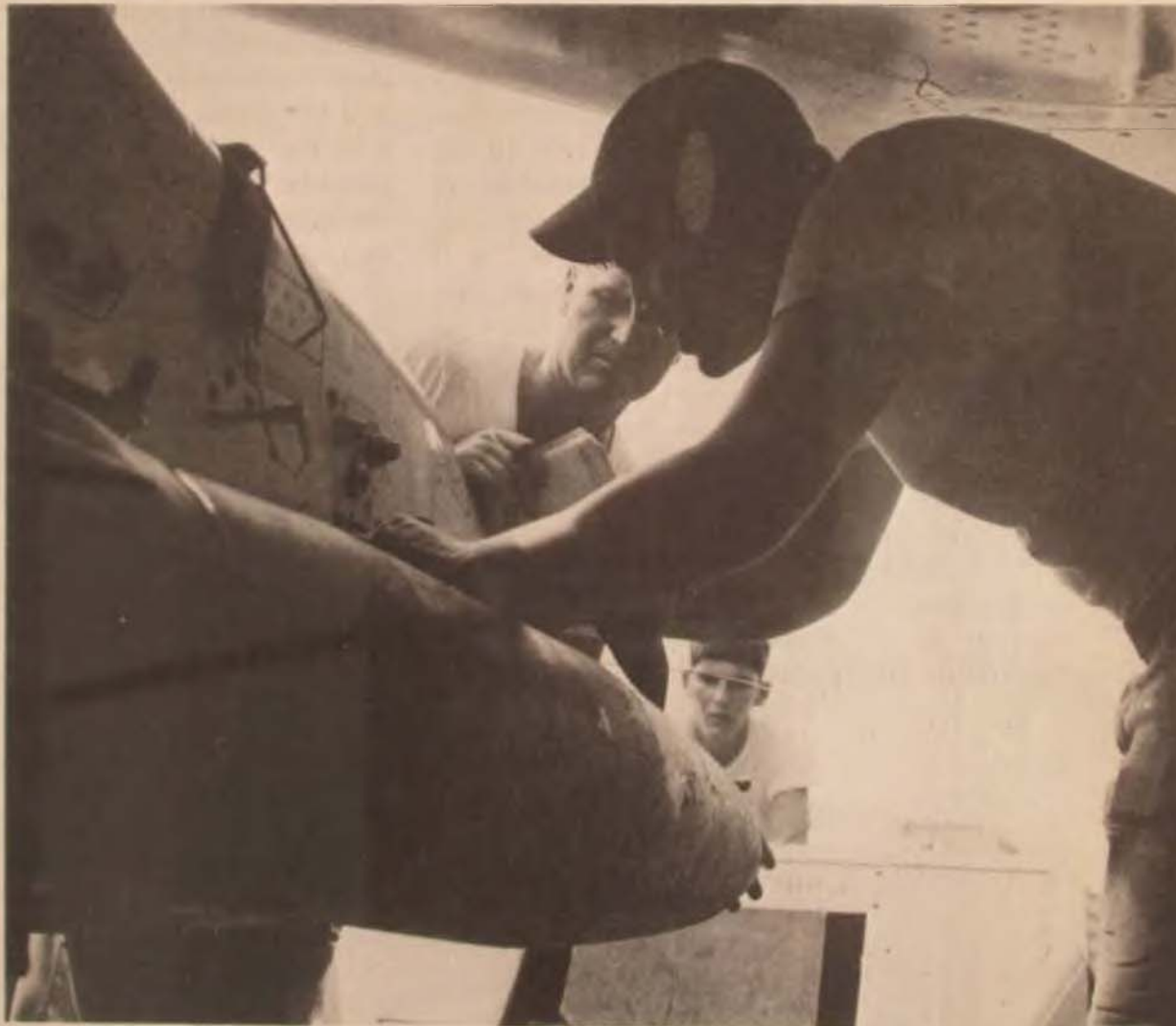
In Vietnam, after the maintenance technicians have finished their work, armament specialists add the decisive payload—like a 500-pound bomb attached to the bomb rack of an F-4C.
